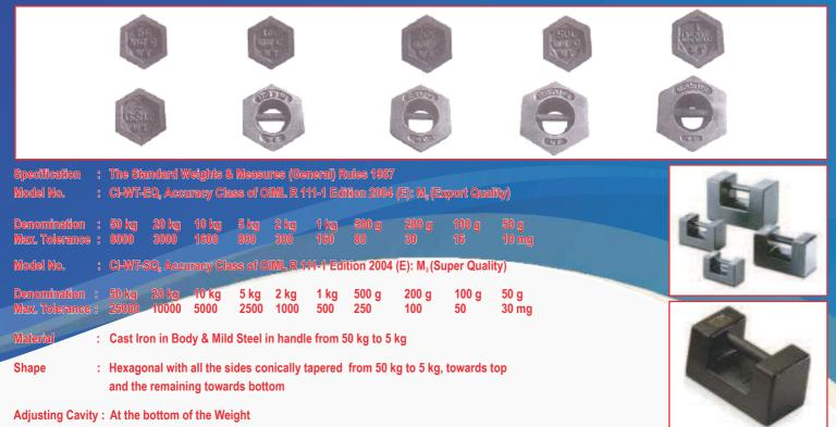
OIML recommended the above vide R-52 Edition 2004(E), for normal use in Trade and Commerce, Cast Iron Hexagonal Standard Weights from 50 g, 100 g, 200 g, 500 g, 1 kg, 2 kg, 5 kg, 10 kg, 20 kg and 50 kg. These can be stacked conventionally and re-verified or re-adjusted periodically. The control mark as required by law is placed on the lead cast in the adjusting cavity. 2 kg to 50 g with nesting arrangement and 50 kg to 5 kg having the handle & a wide circular clear hole for easy lifting.
